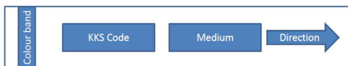
Figure 31: Non-lagged Piping Greater than 50mm
